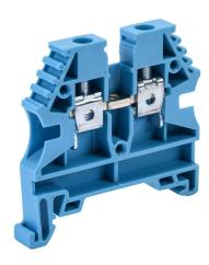
Konnect-It screw single-level feedthrough terminal block, accepts wire size 26-10 AWG, blue, 30A, 35mm DIN rail mount, 100kA SCCR. Package of 20. For use with jumpers KN-2J10, KN-3J10, KN-4J10 and KN-10J10.
