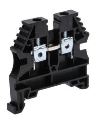
Konnect-It screw single-level feedthrough terminal block, accepts wire size 26-10 AWG, black, 30A, 35mm DIN rail mount, 100kA SCCR. Package of 80. For use with jumpers KN-2J10, KN-3J10, KN-4J10 and KN-10J10.
