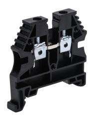
Konnect-It screw single-level feedthrough terminal block, accepts wire size 26-10 AWG, black, 30A, 35mm DIN rail mount, 100kA SCCR. Package of 20. For use with jumpers KN-2J10, KN-3J10, KN-4J10 and KN-10J10.
