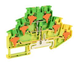
Konnect-It screwless grounding terminal block, triple-level connected between levels, accepts wire size 28-12 AWG, yellow/green, 300 VAC/VDC, 35mm DIN rail mount. Package of 50.
