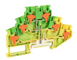
Konnect-It screwless grounding terminal block, triple-level connected between levels, accepts wire size 28-12 AWG, yellow/green, 300 VAC/VDC, 35mm DIN rail mount. Package of 25.
