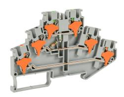
Konnect-It screwless feedthrough terminal block, triple-level, power indicator between levels 2 and 3, accepts wire size 28-12 AWG, gray, 20A, 48 VAC/VDC, LED indicator(s), 35mm DIN rail mount. Package of 25.
