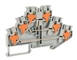
Konnect-It screwless feedthrough terminal block, triple-level, power indicator between levels 2 and 3, accepts wire size 28-12 AWG, gray, 20A, 24 VAC/VDC, LED indicator(s), 35mm DIN rail mount. Package of 25.
