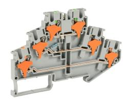
Konnect-It screwless feedthrough terminal block, triple-level, power indicator between levels 2 and 3, accepts wire size 28-12 AWG, gray, 20A, 220 VAC/VDC, LED indicator(s), 35mm DIN rail mount. Package of 50.
