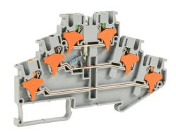
Konnect-It screwless feedthrough terminal block, triple-level, power indicator between levels 2 and 3, accepts wire size 28-12 AWG, gray, 20A, 220 VAC/VDC, LED indicator(s), 35mm DIN rail mount. Package of 25.
