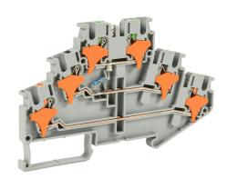
Konnect-It screwless feedthrough terminal block, triple-level, power indicator between levels 2 and 3, accepts wire size 28-12 AWG, gray, 20A, 110 VAC/VDC, LED indicator(s), 35mm DIN rail mount. Package of 50.
