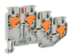
Konnect-It screwless feedthrough terminal block, triple-level, sensor PNP power indicator, accepts wire size 28-12 AWG, gray, 20A, 24 VAC/VDC, LED indicator(s), 35mm DIN rail mount. Package of 50.
