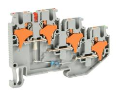
Konnect-It screwless feedthrough terminal block, triple-level, sensor NPN power indicator, accepts wire size 28-12 AWG, gray, 20A, 24 VAC/VDC, LED indicator(s), 35mm DIN rail mount. Package of 25.
