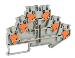
Konnect-It screwless feedthrough terminal block, triple-level, connected between levels 2 and 3, accepts wire size 28-12 AWG, gray, 20A, 300 VAC/VDC, 35mm DIN rail mount. Package of 50.
