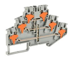
Konnect-It screwless feedthrough terminal block, triple-level, connected between all levels, accepts wire size 28-12 AWG, gray, 20A, 300 VAC/VDC, 35mm DIN rail mount. Package of 50.
