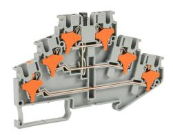
Konnect-It screwless feedthrough terminal block, triple-level, connected between levels two and three, accepts wire size 28-12 AWG, gray, 20A, 300 VAC/VDC, 35mm DIN rail mount. Package of 25.
