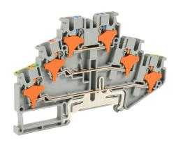
Konnect-It screwless feedthrough terminal block, triple-level with ground and marked for phase neutral and ground, accepts wire size 28-12 AWG, gray, 20A, 300 VAC/VDC, 35mm DIN rail mount. Package of 50.
