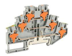
Konnect-It screwless feedthrough terminal block, triple-level with ground, accepts wire size 28-12 AWG, gray, 20A, 300 VAC/VDC, 35mm DIN rail mount. Package of 50.
