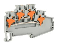
Konnect-It screwless compact feedthrough terminal block, double-level, accepts wire size 28-12 AWG, gray, 20A, 150 VAC/VDC, 35mm DIN rail mount. Package of 50.
