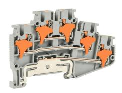
Konnect-It screwless compact feedthrough terminal block, double-level with ground, accepts wire size 28-12 AWG, gray, 20A, 150 VAC/VDC, 35mm DIN rail mount. Package of 50.
