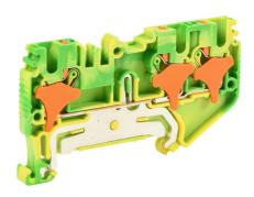
Konnect-It screwless grounding terminal block, single-level, 2 inputs to 1 output, accepts wire size 28-12 AWG, yellow/green, 600 VAC/VDC, 35mm DIN rail mount. Package of 25.
