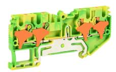
Konnect-It screwless grounding terminal block, single-level, 2 inputs to 2 outputs, accepts wire size 28-12 AWG, yellow/green, 600 VAC/VDC, 35mm DIN rail mount. Package of 50.
