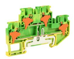
Konnect-It screwless grounding terminal block, double-level connected between levels, accepts wire size 28-12 AWG, yellow/green, 300 VAC/VDC, 35mm DIN rail mount. Package of 50.
