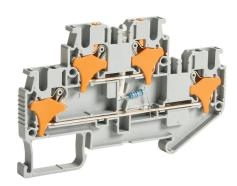
Konnect-It screwless feedthrough terminal block, double-level, connected between levels with power indicator, accepts wire size 28-12 AWG, gray, 20A, 220 VAC/VDC, LED indicator(s), 35mm DIN rail mount. Package of 25.
