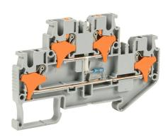
Konnect-It screwless feedthrough terminal block, double-level, connected between levels with power indicator, accepts wire size 28-12 AWG, gray, 20A, 110 VAC/VDC, LED indicator(s), 35mm DIN rail mount. Package of 25.
