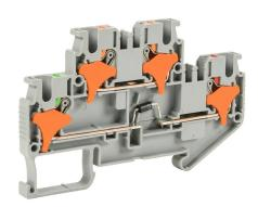
Konnect-It screwless feedthrough terminal block, double-level, 1 diode connected lower level, cathode on input, accepts wire size 28-12 AWG, gray, 1A, 300 VAC/VDC, 35mm DIN rail mount. Package of 25.
