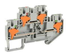
Konnect-It screwless feedthrough terminal block, double-level, 2 diodes connected between levels, lower level no connection, cathodes on top level, accepts wire size 28-12 AWG, gray, 1A, 300 VAC/VDC, 35mm DIN rail mount. Package of 25.
