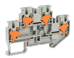
Konnect-It screwless feedthrough terminal block, double-level, 1 diode connected between levels, 1 diode on lower level, cathodes on output, accepts wire size 28-12 AWG, gray, 1A, 300 VAC/VDC, 35mm DIN rail mount. Package of 25.
