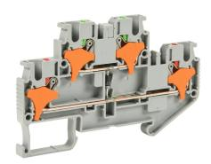
Konnect-It screwless feedthrough terminal block, double-level, 1 diode connected between levels, cathode on lower level, accepts wire size 28-12 AWG, gray, 1A, 300 VAC/VDC, 35mm DIN rail mount. Package of 25.
