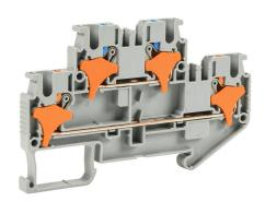
Konnect-It screwless feedthrough terminal block, double-level, marked for phase and neutral, accepts wire size 28-12 AWG, gray, 20A, 300 VAC/VDC, 35mm DIN rail mount. Package of 25.
