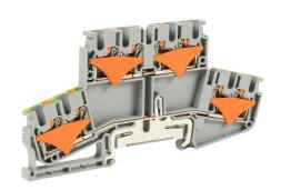
Konnect-It screwless feedthrough terminal block, double-level, 4 inputs to 4 outputs with ground, accepts wire size 28-12 AWG, gray, 20A, 300 VAC/VDC, 35mm DIN rail mount. Package of 50.
