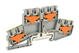
Konnect-It screwless feedthrough terminal block, double-level, 4 inputs to 4 outputs with ground, accepts wire size 28-12 AWG, gray, 20A, 300 VAC/VDC, 35mm DIN rail mount. Package of 25.
