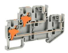
Konnect-It screwless feedthrough terminal block, double-level, pin connection input, accepts wire size 28-12 AWG, gray, 10A, 150 VAC/VDC, 35mm DIN rail mount. Package of 50.
