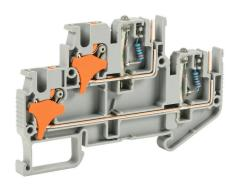
Konnect-It screwless feedthrough terminal block, double-level, pin connection input with power indicator, accepts wire size 28-12 AWG, gray, 10A, 24 VAC/VDC, LED indicator(s), 35mm DIN rail mount. Package of 25.
