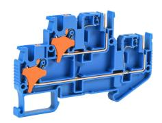
Konnect-It screwless feedthrough terminal block, double-level, pin connection input, accepts wire size 28-12 AWG, blue, 10A, 150 VAC/VDC, 35mm DIN rail mount. Package of 50.
