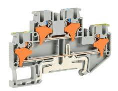
Konnect-It screwless feedthrough terminal block, double-level with ground and marked for neutral and ground, accepts wire size 28-12 AWG, gray, 20A, 300 VAC/VDC, 35mm DIN rail mount. Package of 50.
