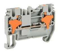
Konnect-It screwless feedthrough terminal block, single-level, accepts wire size 28-12 AWG, gray, 20A, 600 VAC/VDC, 35mm DIN rail mount. Package of 100.
