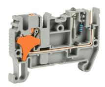
Konnect-It screwless feedthrough terminal block, single-level, pin connection input power indicator, accepts wire size 28-12 AWG, gray, 10A, 24 VAC/VDC, LED indicator(s), 35mm DIN rail mount. Package of 50.
