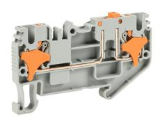
Konnect-It screwless disconnect terminal block, single-level disconnect, accepts wire size 28-12 AWG, gray, 20A, 300 VAC/VDC, 35mm DIN rail mount. Package of 25.
