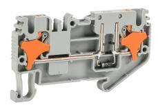
Konnect-It screwless feedthrough terminal block, single-level, 1 input to 1 output with diode, cathode on output, accepts wire size 28-12 AWG, gray, 1A, 300 VAC/VDC, 35mm DIN rail mount. Package of 25.
