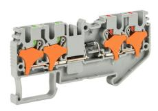
Konnect-It screwless common point feedthrough terminal block, single-level, 2 inputs to 2 outputs bridged with diode, cathode on input, accepts wire size 28-12 AWG, gray, 1A, 600 VAC/VDC, 35mm DIN rail mount. Package of 50.
