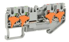
Konnect-It screwless common point feedthrough terminal block, single-level, 2 inputs to 2 outputs bridged with diode, cathode on input, accepts wire size 28-12 AWG, gray, 1A, 600 VAC/VDC, 35mm DIN rail mount. Package of 25.
