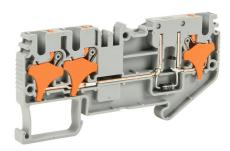
Konnect-It screwless common point feedthrough terminal block, single-level, 1 input to 2 outputs with diode, cathode on input, accepts wire size 28-12 AWG, gray, 1A, 300 VAC/VDC, 35mm DIN rail mount. Package of 50.
