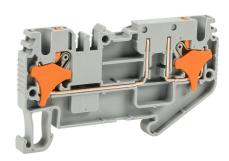
Konnect-It screwless feedthrough terminal block, single-level, bridged disconnect, accepts wire size 28-12 AWG, gray, 20A, 300 VAC/VDC, 35mm DIN rail mount. Package of 25.
