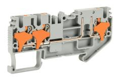
Konnect-It screwless common point feedthrough terminal block, single-level, 1 input to 2 outputs bridged, accepts wire size 28-12 AWG, gray, 20A, 300 VAC/VDC, 35mm DIN rail mount. Package of 50.
