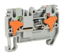
Konnect-It screwless feedthrough terminal block, single-level with diode, cathode on input, accepts wire size 28-12 AWG, gray, 1A, 600 VAC/VDC, 35mm DIN rail mount. Package of 50.
