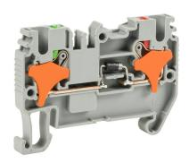
Konnect-It screwless feedthrough terminal block, single-level with diode, cathode on input, accepts wire size 28-12 AWG, gray, 1A, 600 VAC/VDC, 35mm DIN rail mount. Package of 25.
