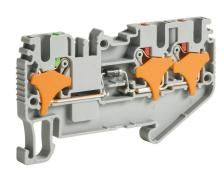
Konnect-It screwless common point feedthrough terminal block, single-level, 2 inputs to 1 output with diode, cathode on input, accepts wire size 28-12 AWG, gray, 1A, 600 VAC/VDC, 35mm DIN rail mount. Package of 50.
