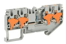
Konnect-It screwless common point feedthrough terminal block, single-level, 2 inputs to 2 outputs bridged with power indicator, accepts wire size 28-12 AWG, gray, 20A, 24 VAC/VDC, LED indicator(s), 35mm DIN rail mount. Package of 50.
