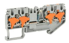
Konnect-It screwless common point feedthrough terminal block, single-level, 2 inputs to 2 outputs bridged with power indicator, accepts wire size 28-12 AWG, gray, 20A, 24 VAC/VDC, LED indicator(s), 35mm DIN rail mount. Package of 25.
