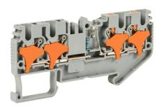
Konnect-It screwless common point feedthrough terminal block, single-level, 2 inputs to 2 outputs bridged with power indicator, accepts wire size 28-12 AWG, gray, 20A, 220 VAC/VDC, LED indicator(s), 35mm DIN rail mount. Package of 50.
